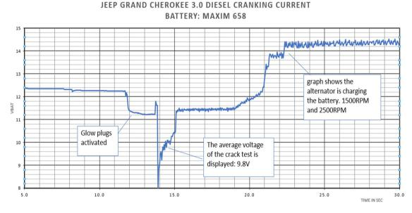
After the engine has started, it is useful to increase the engine's RPMs to observe the difference in the alternator/regulator performance, especially for older cars which have less sophisticated electronic battery charging methods. The graph above shows the alternator/regulator is operating correctly.
