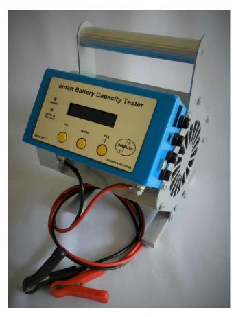
The discharge current can be selected between 1A and maximum for that battery voltage. Refer to the specification section below for details. The unit will log the battery voltage to a unique file on the SD card every minute. The filename is clearly displayed and it must be noted with that specific battery. Upon completion, the display will show the tested battery capacity in Ah.
